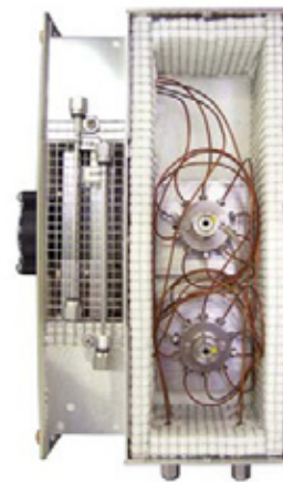
Dual TO-14 Concentrator (four traps, two valves)
